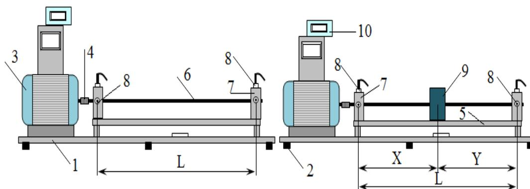
**Figure 1.** Schematic diagram of experimental apparatus: (1) Base; (2) Rubber isolators; (3) Motor; (4) Coupling; (5) Extended rotor deck; (6) Shaft; (7) Bearing housing; (8) Accelerometer; (9) Disk; (10) Tachometer.
